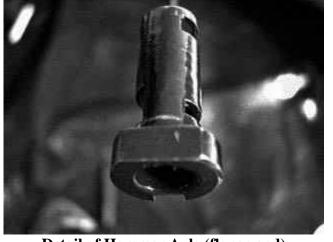
Detail of Hammer Axle (flange end)
