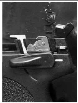
**Detent Plate partially removed**
