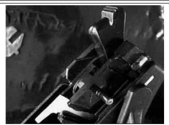
Detail of Sear Axle partially removed
