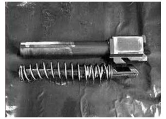
Correct Barrel to Recoil/Buffer Spring Assembly
