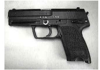
Slide in forward Position and Hammer De-Cocked
