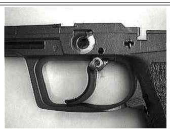
Detail of Trigger rotated forward and partially removed
