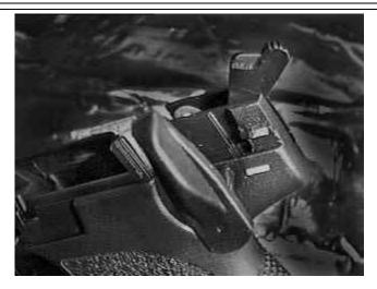
12. Press down slightly on the Trigger Bar and remove the Hammer Axle using a pair of tweezers.
