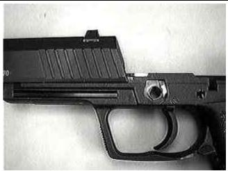
Detail of the Slide just prior to engaging first Slide Inserts (note the Slide Release Shaped Spring just to the rear of the Slide Release Lever axle hole)
