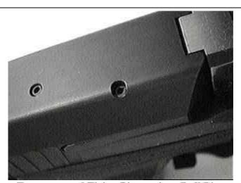
**Extractor and Firing Pin retainer Roll Pins**
