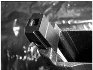
**Lanyard Loop Insert prior to Pin reinstallation**
