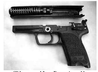
**Slide removed from Frame Assembly**
