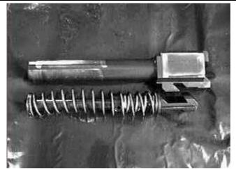
Correct Barrel to Recoil/Buffer Spring Assembly orientation
