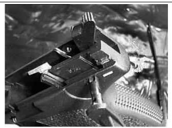
**Detail of Control Lever pulled out**
