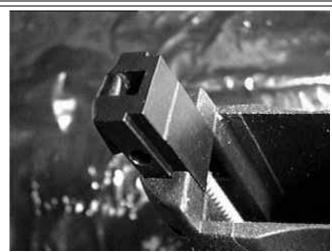
**Lanyard Loop Insert with Pin removed**
