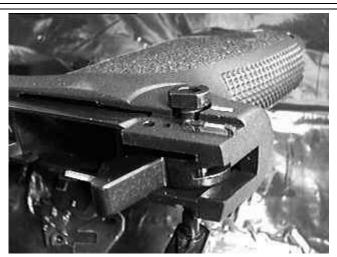
Hammer Axle partially removed (note the flat is facing upwards)
