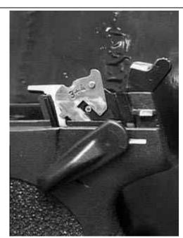
**Detent Plate almost completely removed**
