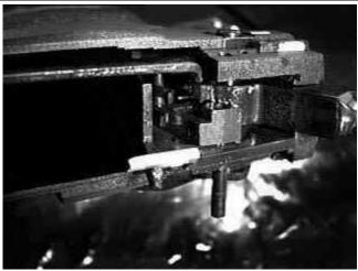
Detail of the Sear in installed position (the Sear Axle is installed just far enough to engage the left wall of the Frame and the Sear only)
