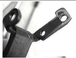
Detail of the back side of the Trigger to Trigger Bar pivot point
