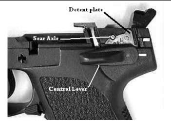
Detail of Control Lever and Detent Plate and Sear Axle.
