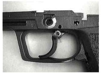
**Detail of Trigger partially installed**
