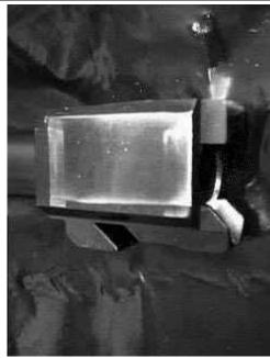
Detail of Barrel Locking Block/Feed Ramp area
