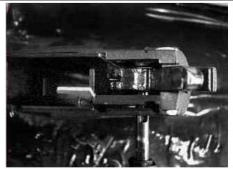
**Detail of Hammer in installed location**
