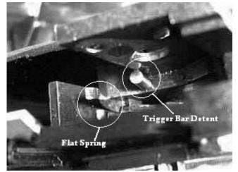
Detail view of the Flat Spring (left) and the Trigger Bar Detent (right)
