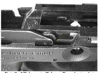
Detail of Trigger to Trigger Bar pivot point
