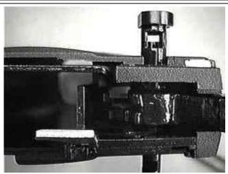
**Detail of the Hammer Axle being installed**
