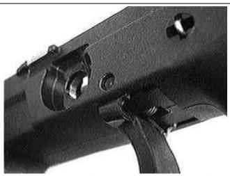
Detail of Trigger, Spring, and Axle viewed from below (note rearward spring end is on back of Trigger)
