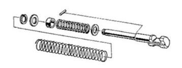
Exploded View of the Recoil/Buffer Spring Assembly
