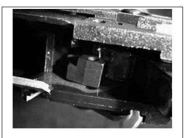
11. Rotate the Control Lever to 12 o'clock, press the Trigger Bar down slightly, then pull the Control Lever out to the left as far as it will go (you may hear a click). You do not need to remove the Control Lever at this time.
