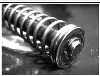
Detail of Guide Rod end, Spring, Retainer, and Snap-Ring on "captured" Recoil/Buffer Spring Assembly
