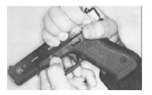
If the slide is drawn back too far (more than 3mm), the trigger will move to the foremost forward position. The slide will then **not** separate from the receiver (17). **Do not use force**. The trigger must first be pulled all the way back.
