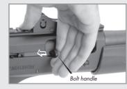
During this operation, any shell present in the chamber will be ejected. Avoid damage to the shell by not letting it fall on hard ground.
