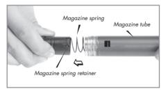
Let the magazine follower (refer to photo in § 5.6) slide out of the magazine tube by inclining the shotgun as necessary.
