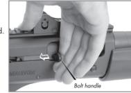
During this operation, any shell present in the chamber will be ejected. Avoid damage of the shell by not letting it fall on hard ground.
