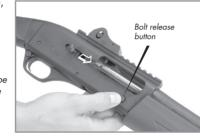
Keep your fingers away from the ejection opening when using the bolt release button to close the action!
