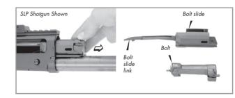
Separate the bolt and the bolt slide.
