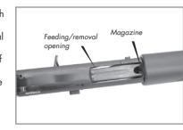
If there is a shell in the chamber and/or magazine, try to extract and eject it by successively closing and opening the bolt.
