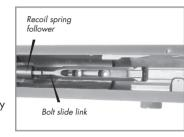
The recoil spring follower can be seen at the rear side of the cavity in the bottom of the receiver.
