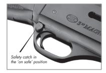
The above diagram shows a right-hand safety catch. The 'on safe' position is with the catch pushed to the right.
