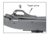
This level of disassembly of the trigger group is sufficient to perform thorough cleaning. Further disassembly should only be carried out by an authorized armorer or by FN HERSTAL.
