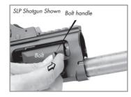
The bolt handle should be oriented so that its ribbed side is facing forward.
