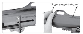
The two trigger group positioning pins can be removed from either side of the receiver.
