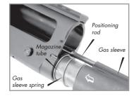
The gas sleeve should be oriented so that its positioning rod is at the rear side and the positioning rod of the gas sleeve should fit into its housing provided in the left front side of the receiver, just underneath the opening for the barrel.
