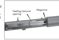
If a shell remains in the chamber and/or magazine, try to extract and eject it by successively closing and opening the bolt.
