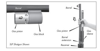
While holding the shotgun at the vertical position, install the assembly formed by the barrel and the gas piston onto the front part of the gun.
