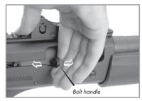
Keep your fingers away from the ejection opening when releasing the bolt handle to close the bolt!
