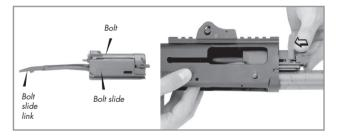
Partly insert the assembly formed by the bolt and the bolt slide, with the link of the bolt slide first, into the front part of the receiver.
