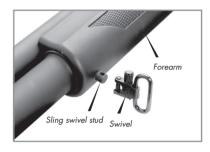
If desired, fix a sling swivel to the sling stud provided underneath the buttstock of the shotgun.
