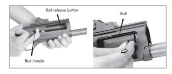
Ensure that the bolt is released and then gently guide the bolt slowly and carefully forward until it rests at its front position.
