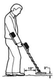
Adjust the stem length and coil angle so the coil rests flat on the ground about 6 to 12 inches in front of your foot. Move into your "search" position by leaning slightly and raising the coil about 2 inches off the ground. This should put the coil about 12 to 18 inches in front of your lead foot.
