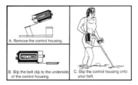
The Gold Bug control housing can be hipmounted to reduce weight on the stem and create nearly effortless hunting. Belt loops are provided on the underside of the control housing.
