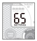
When the SETTING value represents the Ground Balance setting, "GND BAL" will be displayed next to the number.
