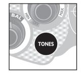
In <u>All-Metals mode</u>, the TONES button allows the user to vary the pitch of the base tone.
