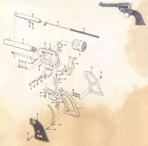
LOADING. Draw the hammer back to the Half-Cock position. Do not touch the trigger but leave it free to snap into the notch. (NOTE: If the hammer should be at the Full-Cock position, lower it all the way first and then draw back to Half-Cock. Otherwise, the bolt cam lever cannot operate to release the cylinder.) This will leave the cylinder free to rotate for loading. Open the Loading Gate on the right-hand side of the revolver and load each chamber. Close the loading gate.
