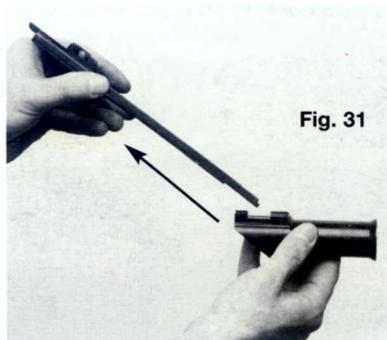
The trigger group may be removed from the receiver for further cleaning of the receiver and trigger group. It is recommended that a thorough cleaning be performed every 300 rounds.
