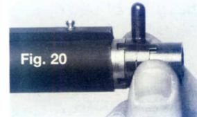
Your VR-MC barrel is threaded for your choke tubes. For internal tubes, insert the wrench into the slotted portion of the tube and turn counterclockwise to remove it from the barrel and turn clockwise to install it. Fig. 20.
