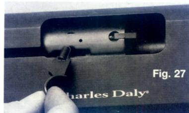
After you remove the bolt handle, the entire action bar/bolt assembly can be removed from the shotgun by pulling the action bar off the end of the magazine tube. See fig. 28.
