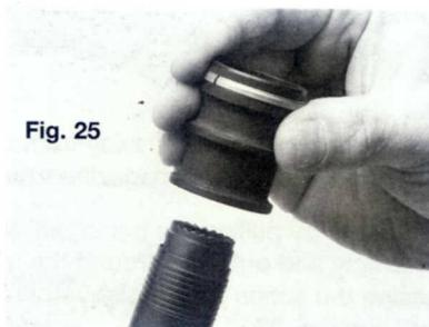
Remove the piston buffer, fig. 26.
