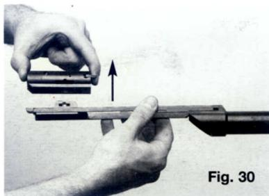
Separate the action bar from the action bar sleeve by pulling the action bar up and away from the action bar sleeve as shown in fig. 31.
