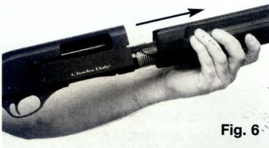
Remove the forend by sliding it forward, off the shotgun as shown in Fig. 7. Note that the forend may be tight to the shotgun when doing this.
