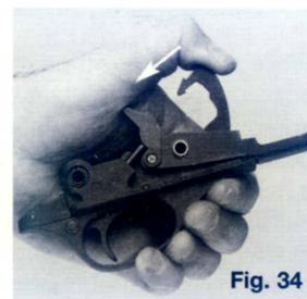
Note: When reinstalling the trigger group, the hammer must be in its cocked position. To cock the hammer, pull down on the hammer with your thumb until it locks into place as shown in fig. 34.
