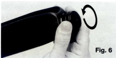
Unscrew the magazine cap from the front of the forend in a counter clockwise direction as shown in Fig. 6.
