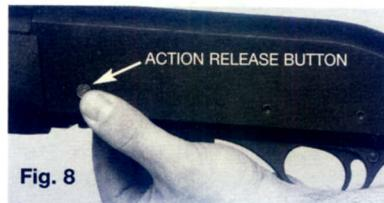
Refer to Fig. 9. While holding the bolt handle with your right hand, depress the action release button with your left thumb and allow the bolt to go forward slowly with your right hand until the bolt handle reaches the end of the receiver.
