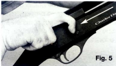
Holding the shotgun as shown in Fig. 5 above, use your finger(s) to pull the bolt handle fully to the rear until the bolt locks in its open position.
