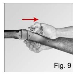
The trigger pressure on your rifle is adjustable on the set trigger assembly. To adjust, screw the trigger adjusting screw inward or outward
