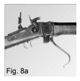
To load the rifle, first point the rifle downrange in a safe direction. Place the rifle on safe by placing the hammer in the half-cock position.
