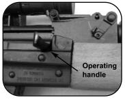
The operating handle is drawn to the rear to check the rifle's loaded/unloaded status.
