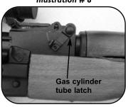
Rotate the gas cylinder tube locking latch upward to free the gas cylinder tube.
