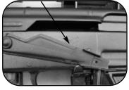
Safety lever in lower or "FIRE" position. Pulling the trigger when the safety lever is in the lower position will result in the rifle firing if there is a round in the chamber! Exercise extreme caution when handling rifle in this condition.
