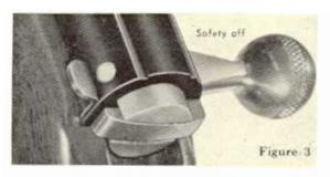
ready to fire. In the OFF SAFE position, a red warning dot is exposed (See Figures 2 & 3). This is a positive safety which locks the trigger and makes it impossible to open the bolt. When the safety is OFF, the rifle cannot fire until the breech bolt is completely forward and locked into position by its cross bolt.
