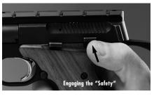
upward into the recess provided for it in the slide (Figure 2). Note: this may require firm pressure. Be sure the lever travels its maximum upward movement and is completely engaged in the recess. Although the sear is now blocked, abusive handling or dropping can cause this or any other firearm to discharge. Be careful when handling any firearm.
