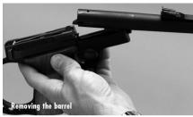
bled Standard Buck Mark (Figure 14). Further disassembly should be performed only by a competent gunsmith or the Browning service facility. Do not remove the grips from the pistol, as they serve to retain and position internal parts.
