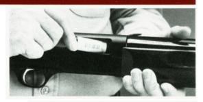
Insert the second cartridge through the loading port at bottom of receiver as shown in Figure 12. Note: MAKE SURE THAT THE CARTRIDGE IS PUSHED PAST THE CARTRIDGE STOP, AND THE CARRIER IS FREE TO MOVE. (See Figure 13.)
