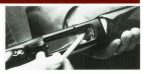
Repeat the above procedure until your gun is fully loaded. Your B-80 will hold three 3 inch or three 2 3/4 inch cartridges in its magazine plus one in its chamber. NOTE: A magazine plug restricting the B-80's magazine capacity to two cartridges is installed at the factory. Instructions for removing the magazine plug will be found on page 42.
