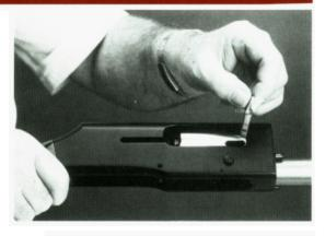
Install the trigger housing, being careful to insert the main spring support into the recess. Depress the cartridge stop and bolt release button. Align all components and replace the trigger assembly retaining pin. (See Figure 26.)
