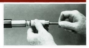
NOTE: The magazine plug is spring loaded and under tension. Be prepared to use both hands in guiding the spring out of, and back into, the magazine tube once the plug has been removed.
