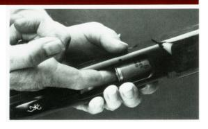
VISUALLY CHECK THE MAGAZINE AND CHAMBER TO MAKE SURE THEY ARE EMPTY. Gather ejected cartridges and store
