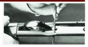
Depress the cartridge stop/bolt release button flush with the receiver and lift the trigger housing forward, up, and out of the receiver. (See Figure 16.)
