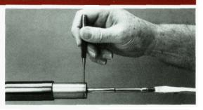
Remove the punch and continue turning the magazine retainer and forearm cap stud until three threads are exposed. At this point lay the screwdriver aside and proceed by hand. (See Figure 28.)
