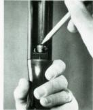
will go all the way back before continuing assembly. If the bolt will not go back freely, remove the assembly and align all components carefully, then repeat procedure.
