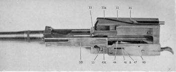
PLATE 9 Internal Mechanism in Backward Position
