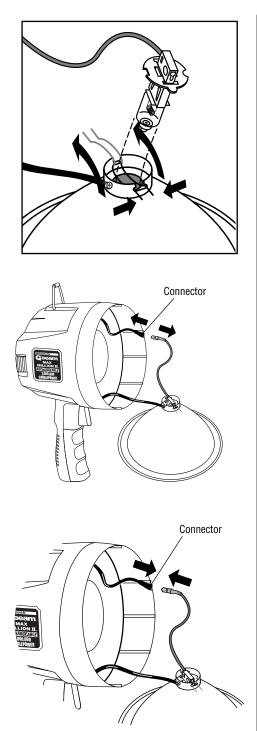
**Step 5:** Holding the front housing secure, slowly lift the rear housing off.
