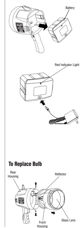
Only use Brinkmann's 12V75W halogen bulb that is designed for the Q-Beam Max Million  ${\rm I\!I}$  Rechargeable spotlight as a replacement. Use of any other bulb may result in poor performance and may damage your spotlight.
