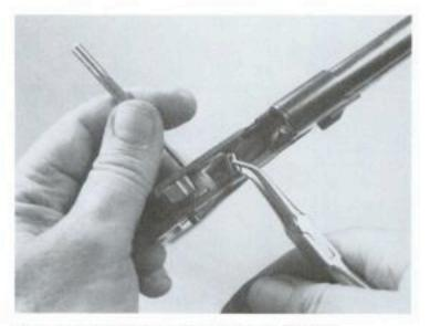
21. Note that when this pin is removed, it will release a cylindrical bushing or spacer that fits between the ejector and the sear trip lever. Take care that this small part isn't lost.
