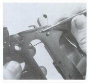
20. Drift out the ejector stabilizer pin toward the right.
