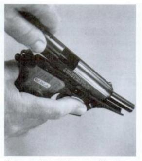
Draw the slide back all the way and lift it up at the rear. The slide can then be moved forward off the barrel and frame, and the recoil spring can be removed from the barrel. Gun is now field-stripped.
