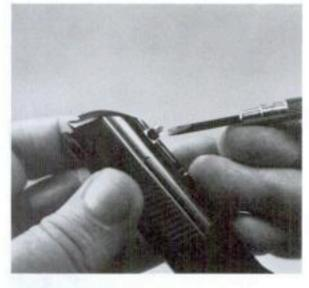
With a non-marring tool, the rear sight can be drifted out of its dovetail toward the right. The sight leaf can be taken out of the base by backing out the adjustment screw. Take care that the small coil spring behind the bottom of the leaf isn't lost.
