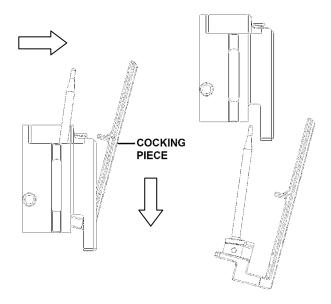
Remove the two firing springs.
