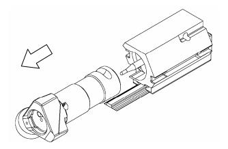
Pivot the cocking piece so that spring retainer clears the bolt carrier, then remove it from the rear of the bolt carrier.
