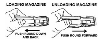
To unload magazine, hold magazine with one hand with the projectile tips facing away from you. Push each of the cartridges out of the magazine until all are ejected.
