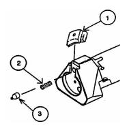
Installation of the extractor is reverse of removal.
