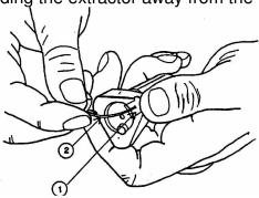
Slide the extractor (1) out of its slot. The extractor spring (2), and extractor plunger (3) can then be removed, but be careful to contain the spring and plunger.
