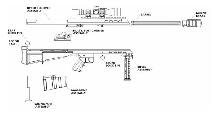
Lock Pins: The lock pins connect the upper and lower receivers. One pin is located forward of the butt, the other in front of trigger group.
