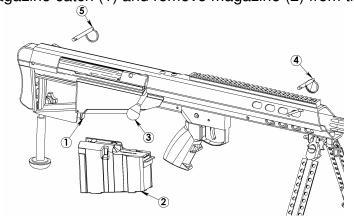
Unlock the bolt (3) by lifting the bolt handle upward and pulling it to the rear. Withdraw the mid lock pin (4) and rear lock pin (5) from the receiver.
