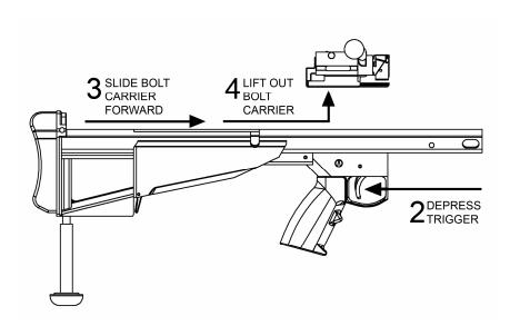
Reassembly is the reverse of disassembly.
