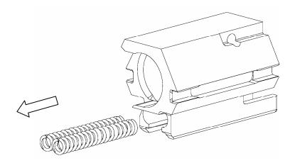
No further disassembly of bolt carrier assembly is necessary.
