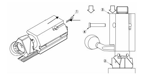
Now remove the bolt from the bolt carrier assembly.
