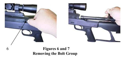
2. Remove the Bolt Group. Unlock the bolt and pull the bolt to the rear of the receiver. Depress the Bolt Catch (6) at the left rear of the Receiver and pull the Bolt Group to the rear and out of the Receiver. Further disassembly of the Bolt Group should be done only for repair or lubrication by a qualified service technician or gun smith.
