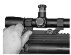
Figure 22 Attaching the ArmaLite Scope Mount
