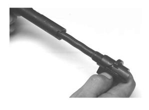
Figures 9 and 10 Removing the Bolt Sleeve and Striker Group
