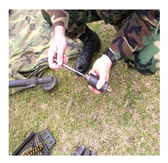
B. Insert each adapter cartridge base-down in the opening of the link positioning tube. Push the adapter cartridge into the link positioning tube to push the cartridge links forward until they stop.
