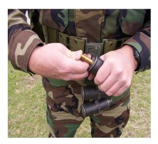
E. The ammunition can is painted blue on the rear to denote that it contains a training device. The opposite (front) of the can is left green to maintain camouflage discipline to the front during training. Insert the loaded belt into the ammunition can with the tips of the cartridges facing front, and with the male end of the belt (the end with the swivel on
