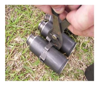
D. Insert an M82 blank into the chamber of each adapter cartridge until it snaps into place and can be pushed no farther. The adapter cartridges have a spring that engages the rim of the blank to hold it in the chamber. The base of the M82 blank should be almost flush with the base of the adapter cartridge.
