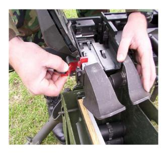
D. Unscrew the AR-22 barrel insert from the yoke.
