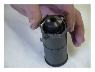
C. Set the link carefully on the cartridge; it must be driven down without tipping or jamming.
