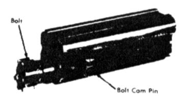
Remove/Install Bolt Com Pin and Bolt Figure 3-15
