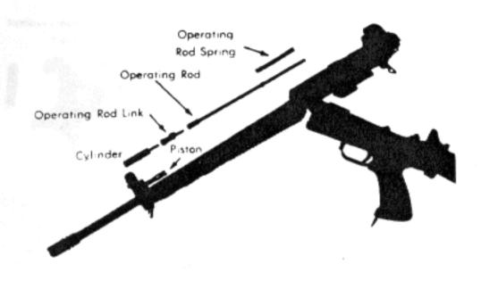
Remove: Install Operating Rod Assembly Figure 3-2
