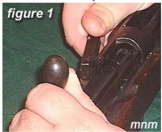
1) Open the bolt stop as show in **figure 1** and remove the **bolt**.
