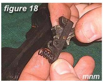
**18) Figure 18** shows the **trigger assembly** with the **spring** correctly installed.
