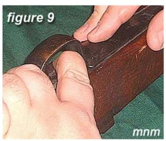
**9)** Press on the **magazine release button** inside the **trigger guard** and open the **magazine cover**.
