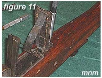
11) Remove the forward trigger guard screw.
