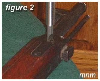
2) Remove the two screws retaining the **forward barrel** bands.
