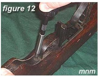
12) Remove the middle trigger guard screw.
