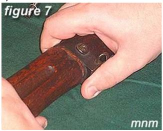
7) Slide the rear barrel band forward.
