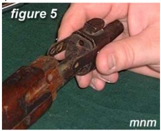
**5)** You will not be able to remove the **barrel bands** without removing the **front sight**. Just leave them attached.
