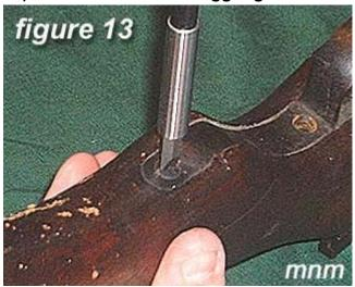
13) Remove the rear trigger guard screw.
