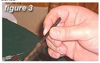
3) Remove the stacking rod by unscrewing it.
