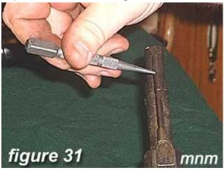
**31)** Use a small punch to insert in hole in front of stacking rod and rotate until tight.
