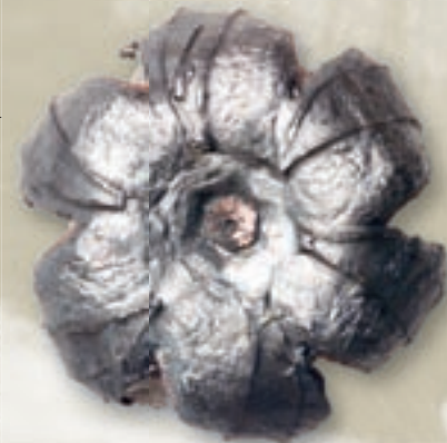
Gold Dot Expanded Bullet. Each Gold Dot bullet is pre-cut at the nose through the jacket and into the core, forming flutes that control expansion on impact.
