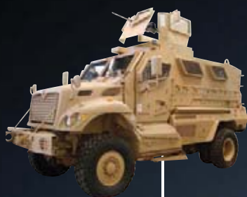
MK19/M240/M249/M2H With O-GPK front gunner shield attached to MK93 mount
