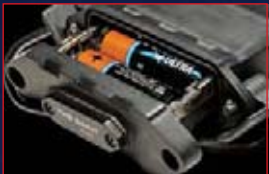
Battery compartment houses 123A lithium or AA alkaline/lithium batteries.
