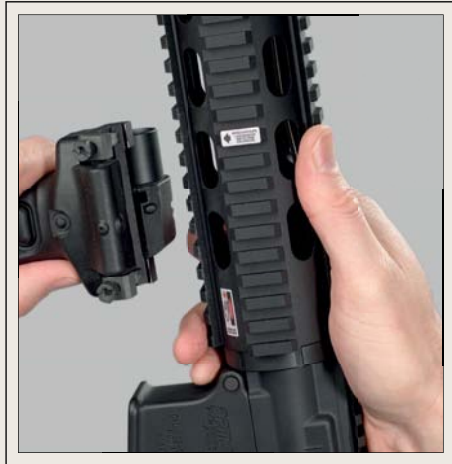
Hold light side at angle lining up lugs to fit into slots in picatinny rail.
