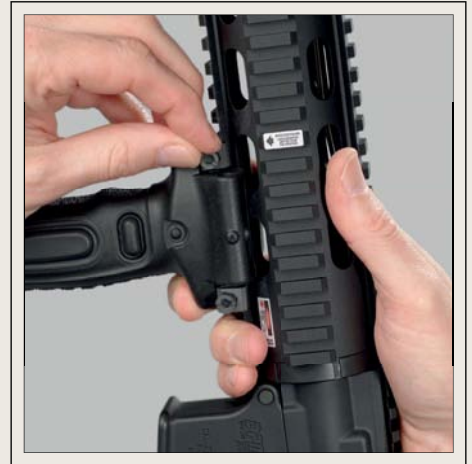
Tighten foregrip onto rail by turning nuts. Use screwdriver or nut driver to tighten. (50-55 inch/lbs.)
