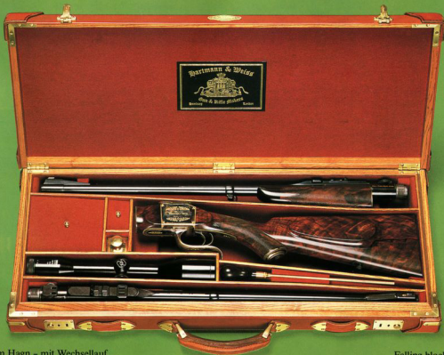
Falling-block rifle - Hagn action - with interchangeable barrel and accessories in case
