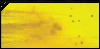
12-gauge 2-3/4" 4B shot at 15 feet gets excellent penetration.
