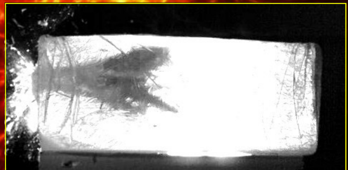
The above block is impacted with an Extreme Shock 9mm 115-grain Enhanced Penetration Round. Note the massive damage channel and fragmentation
