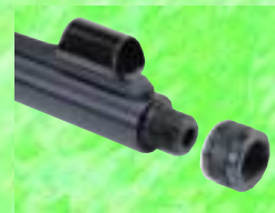
G = Barrel thread.
