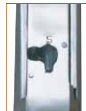
Bolt Mounted Manual Safety on Model 62 and Model 72 Long Guns
