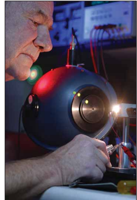
(Light expert) Dr. Peter Hauk runs a test with the integrating sphere photometer in the SureFire laboratory.
