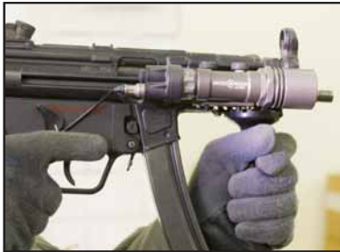
MP5K fitted with SureFire Picatinny rail forend. Attached to rails: an M951 WeaponLight and a vertical foregrip.
