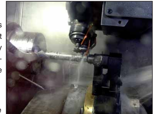
SureFire's Multi-axis Computer Numerically Controlled lathes ensure precision-machined components.
