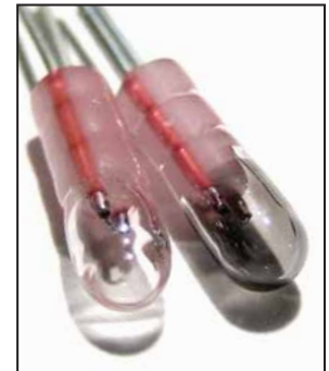
Identical non-SureFire miniature lamps. Left lamp is unused, right lamp shows tungsten deposits after several hours of use.
