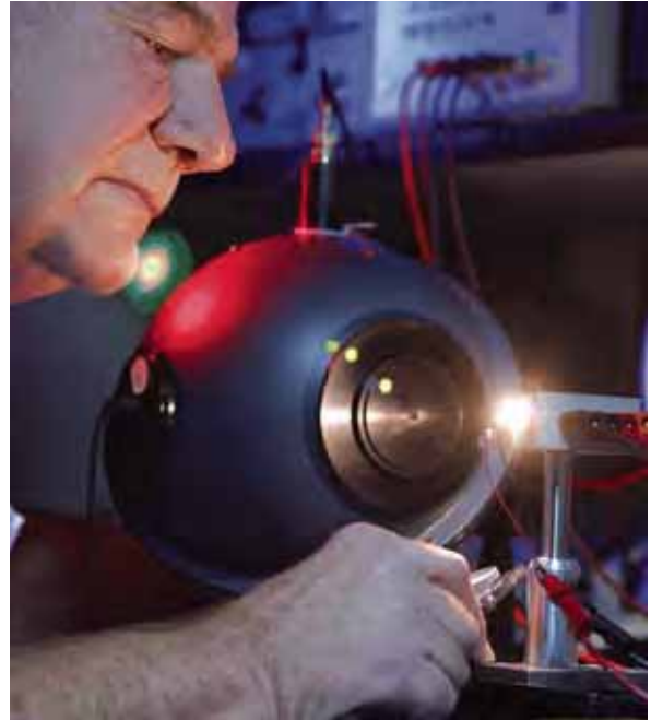
(Light expert) Dr. Peter Hauk runs a test with the integrating sphere photometer in the SureFire laboratory.
