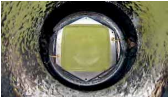
Micro-textured reflector surrounding flat surface of high-output LED.
