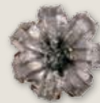
Outstanding Gold Dot performance! Here Gold Dot shows optimum penetration and expansion through Bare Gelatin.
