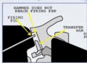
The transfer bar mechanism prevents the hammer from striking the firing pin unless it has been cocked and the trigger pulled rearward.
