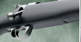
Actions are pillar bedded for strength and accuracy. Twin aluminum pillars are bonded into every stock and support the receiver under guard screw tension and recoil. Match grade triggers set at 3.5–4 pounds break sharp and clean.
