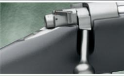
Kimber rifles have a positive, three-position wing safety. The rear position is on safe and locks the bolt, the middle is on safe but unlocks the bolt for loading and unloading, and the forward position permits firing.
