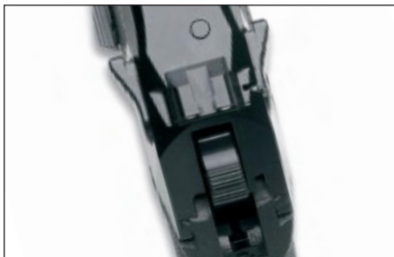
Ambidextrous manual safety (F model).
