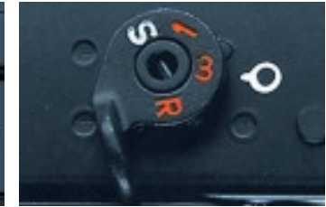
Safety selector lever. (S-1-3-R).
