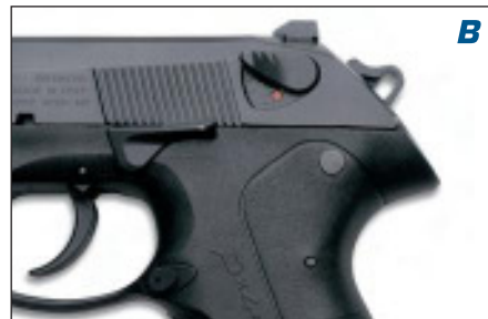
F MODELS. Safety disengaged: A de-cocked hammer. B half-cocked hammer. C cocked hammer. D safety engaged, hammer de-cocked.
