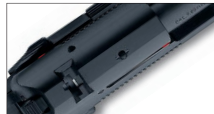
Chamber-loaded indicator. When a round is chambered, the extractor protrudes slightly to show a red indicator. In the dark, the user can feel the protruding indicator.
