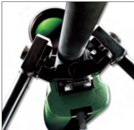
TRG-bipod: especially designed for sniping this new bipod lets the rifle "hang" below the hinge-point offering very steady shooting position even with large and heavy scopes on the rifle.
