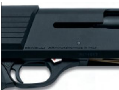
Cut-off device allows replacement of chambered shotshell blocking the feeding
