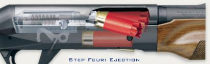
As the empty shell exits the receiver, the energy of the moving bolt assembly recocks the hammer and compresses the recoil spring in the buttstock. The recoil spring then thrusts the bolt assembly forward, lifting the on-coming shell into position and chambering a fresh cartridge. The gun is ready to fire again in a fraction of a second!
