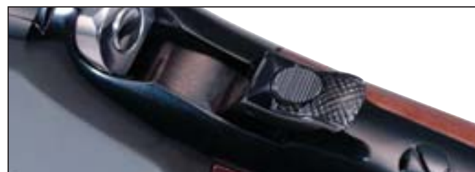
Hammer Mounted Decocker Button on Thunderbolt allows for safer decocking without touching the trigger. The hammer lowers to the intercept notch and stops before striking the firing pin.
