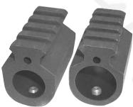
A great addition to both standard and bull barrels, these gas blocks are machined from solid aluminum extrusion. Cut with standard picatinny rails, they will accept all picatinny standard hardware including detachable A-Frame style front sight bases and globe sights. *Please specify the diameter when ordering; (.728") Standard or (.928") Bull diameters.*
