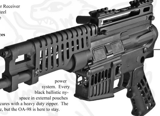
The OA-98 operates off of the OA-93 integrated recoil system and allows the elimination of the buttstock. Looking at the OA-98 you can see that we've taken weight off the pistol wherever it's not needed. A custom mesh handguard, a milled magazine well, and a machined handgrip, all to reduce the weight of this pistol system. The upper receiver is topped with an integrated charging handle and picatinny mounts for custom accessories. The photos also show a maga-
