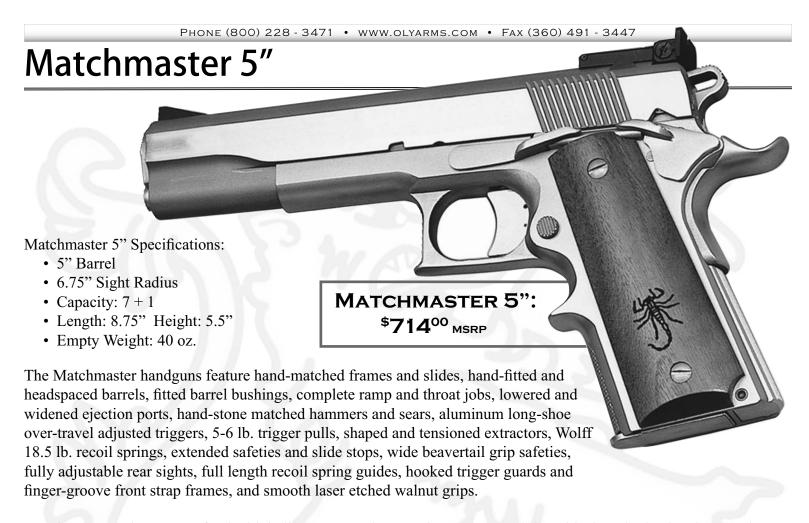
Matchmaster series are test fired with ball, LSWC, and JHP. Choose from stainless, black parkerized carbon, or deuce finish configurations. Also available in a two-tone version known as the "Deuce".
