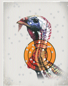
Conventional Turkey Load 1-3/4 oz., #6 lead shot, 1300 fps, 40 yards 13 critical hits, 38 total hits
