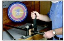
5. Once the headspace is established, the barrel nut is tightened.
