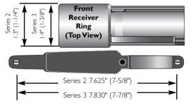
Series 2 (93, 94, 95, 96) — I-1/4" front receiver ring and 7-5/8" center to center on the trigger guard screws. This series includes most Model 93, 94, 95, 96 rifles and carbines.
