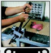
nuts on the 110 and 10 series rifles, and features two 1/2" square drive holes for a swing bar or torque wrench. The Barrel Vise provides plenty of holding force to securely clamp your barrel for removal or installation. The Vise includes two pre-drilled oak blocks, I" and 3/4", and a solid block for custom drilling.
