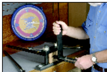
5. Once the headspace is established, the barrel nut is tightened.
