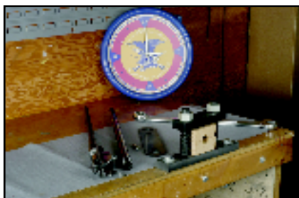
1. The original barreled action, new Adams & Bennett Savage varmint weight barrel, headspace gage, Wheeler Savage Barrel Nut Wrench and Barrel Vise.
