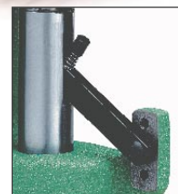
"Smart" primer arm automatically swings into position during the ram stroke and flips out of the way when not in use. For maximum sensitivity at the lowest possible leverage, priming is done at the end of the ram stroke.
