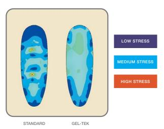
STRESS CONCENTRATION IMAGING showing the behavior of the Gel-Tek pad during the shooting cycle. Note the homogenous distribution of stress over the entire surface.
