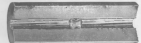
A longitudinal section of the barrel showing pellet lying in the rifled bore.
