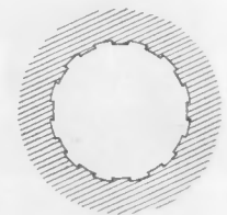
Transverse section showing rifling grooves.
