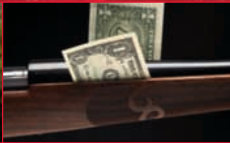
All Model 70s feature free-floating barrels.
