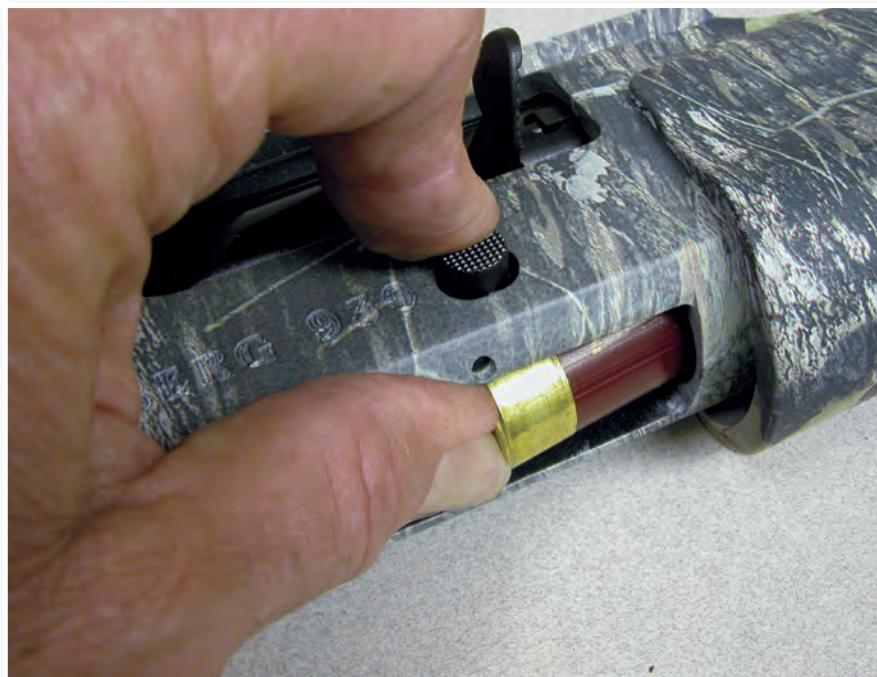
A unique system for unloading the magazine of the 930 allows shells to be removed without cycling through the chamber first.
