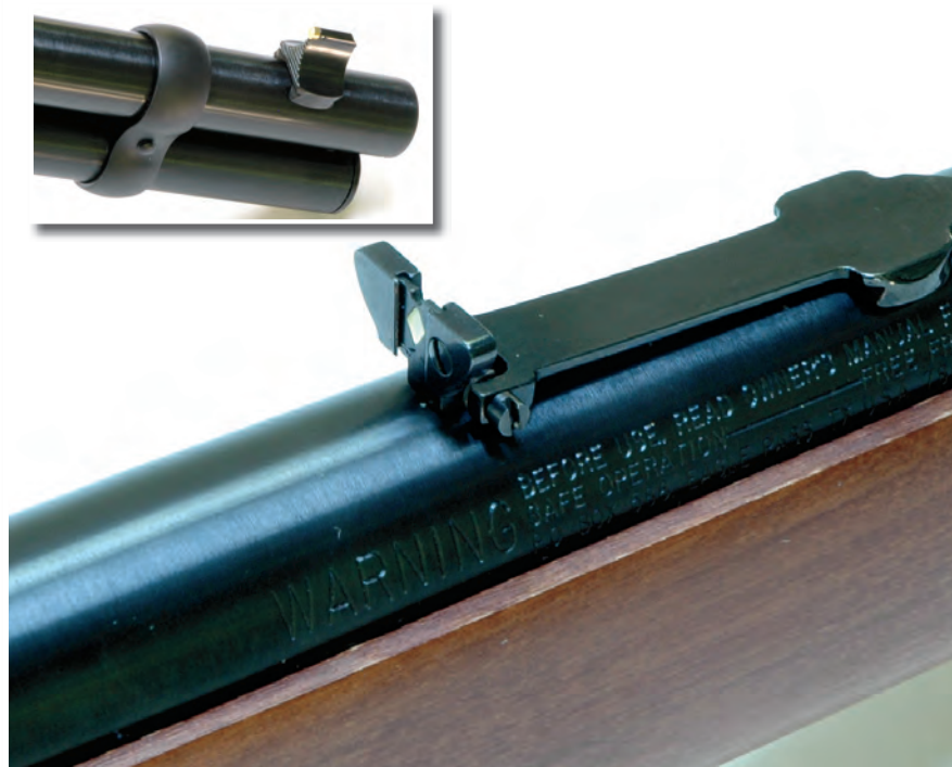
The rear sight is adjustable for elevation and windage and folds to allow low scope mounting; the front is a traditional gold bead.
