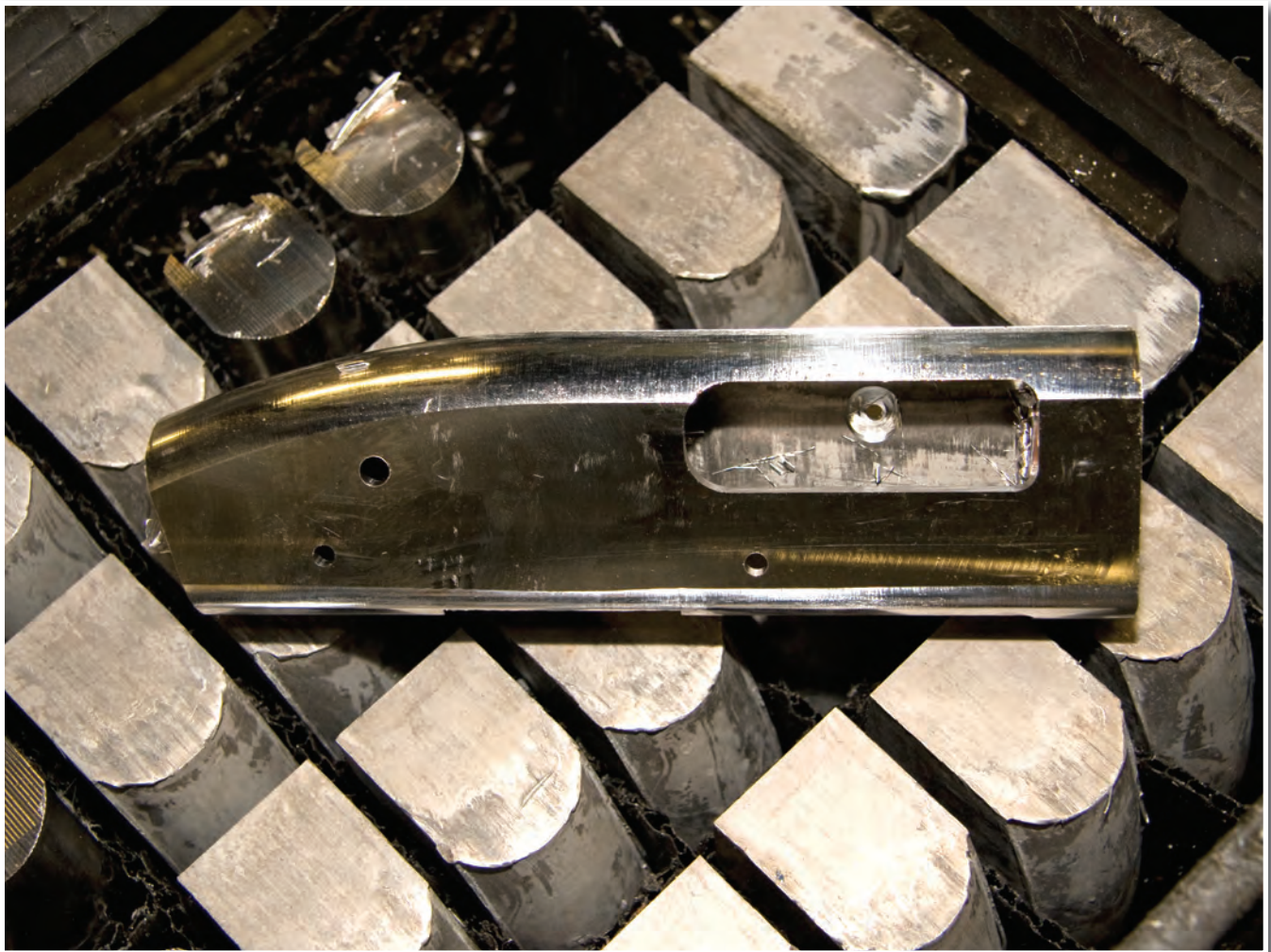
The rugged receivers of the 590A1 are machined from an aluminum forging at Mossberg's North Haven, Connecticut plant.
