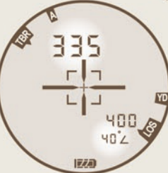
TRUE BALLISTIC RANGE Aim as if the target is 335 yards away
