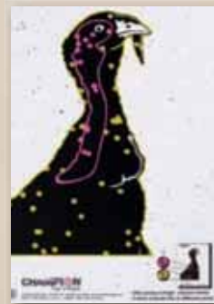
PHT193F 7 with modified choke at 40 yards. Target shot with Rem. 870.
