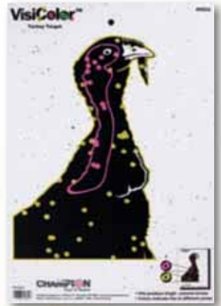
PHT193F 7 with modified choke at 40 yards. Target shot with Rem. 870.
