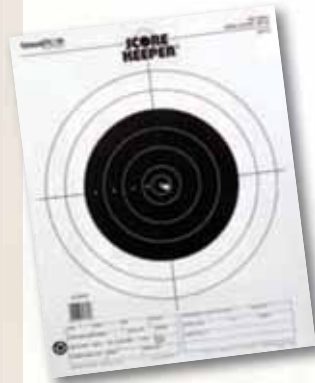
5 shots at 100 yards, 0.164" group center to center (extreme spread) Target shot with UM22 in a Cooper rifle with Weaver® target scope
