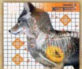
PHC120 BB with full choke at 40 Yards. Target shot with Rem. 1100.
