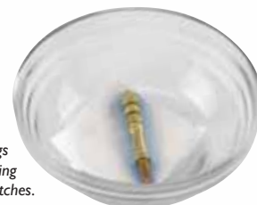
The Ultra Jag shows no sign of copper blueing, even after soaking in bore solvent overnight.
